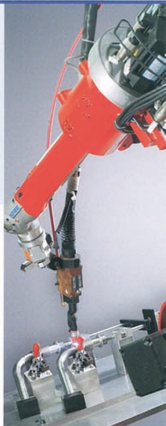
Tacking robot in action
